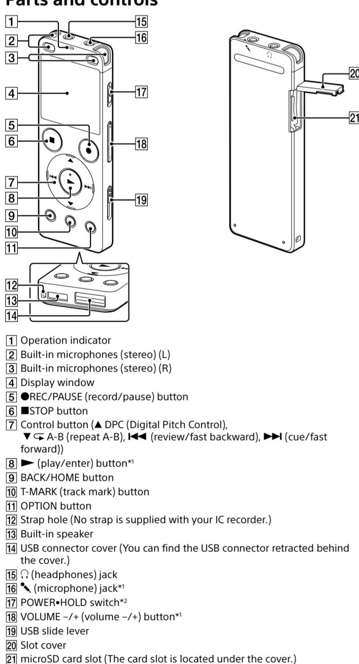
\* The ▶ (play/enter) button, VOLUME -/+ (volume -/+), and (microphone) jack have a tactile dot. Use the tactile dot as a reference when operating the IC recorder.
