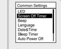
You can keep the display window from turning off or change the default setting to another timer interval. Press and hold BACK/HOME and select "Settings" - "Common Settings" - "Screen Off Timer," and then select "No Auto Screen Off," "15sec," "30sec," "1min," "3min," or "5min."
