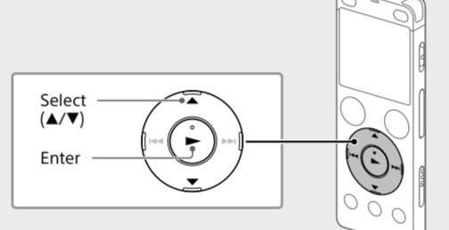
When you turn on your IC recorder for the first time, the "Configure Initial Settings" screen appears on the display window. You can then select the display language, set the clock, and turn on/off the beep sound.
