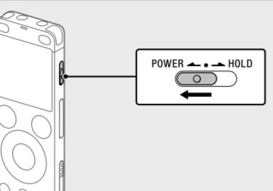
Slide and hold the POWER+HOLD switch in the direction of "POWER" until the window display appears. To turn the power off, slide the POWER+HOLD switch to "POWER" and hold it until "Power Off" appears on the display window.
